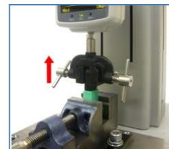
USB connector extracting/inserting force test
