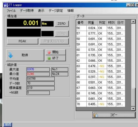
Torque measurement of rotary switch
