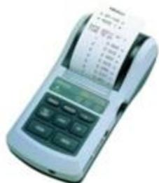
It can print displayed value and inner memory data on the spot. (Required cable:CB-301)
