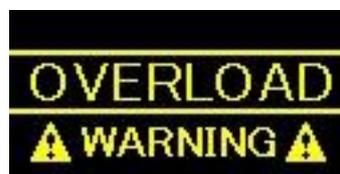
When load over its capacity is added, warning is indicated. Please stops measurement immediately when this indication show up.
