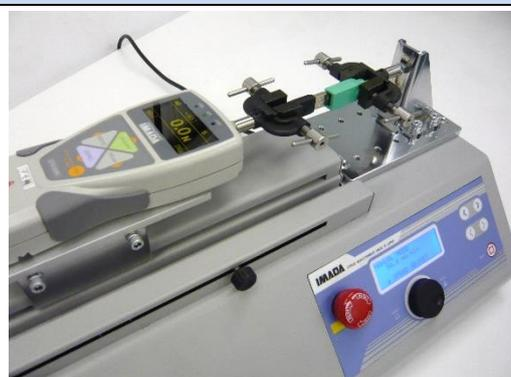
USB connector extraction / insertion (repetition) test
