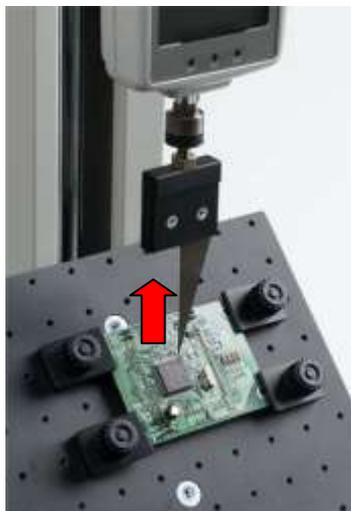
Pull QFP lead with hook on the board of 45 degrees for strength test.
