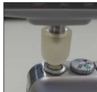
Camera shutter button feeling test
