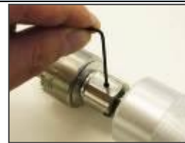
Turn screw by attached L wrench
