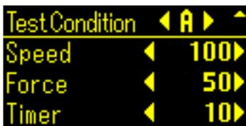
Set the test condition at "Keep loading more than 50N for 10 sec when pulling at 100mm/min".
