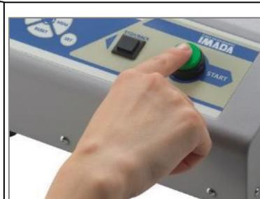
After sample breaking or after loading setting force in setting time, automatically, the moving part is back to the first position.
