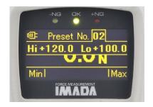
▲ Each preset has a number, so it is possible to instruct the measurement condition by the number. In addition, each measured data has a history of which number preset is used.
