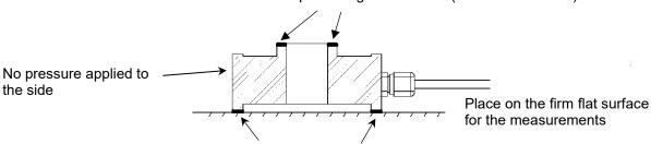
The force applied from the top received at the bottom rim section
