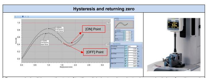
For example, in click sensation test of tactile switch, hysteresis and returning zero is obvious from the graph of a reciprocating motion. It is simple to evaluate the graph by setting threshold value, searching for returning peak values and inserting an arbitrary border line. Moreover, the point of switch ON/OFF can be automatically defined and displayed by using Mark On function.
