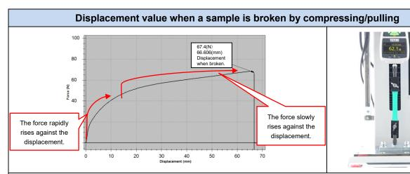
This unit graphs the process and enables you to visually check the force transition until the sample is broken. Also, it helps you to easily find the force/displacement value and peak value when the sample is broken, and leave a comment.
