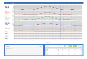
Displays measurement values for all channels in realtime. Continuous data recorded and graphed at 2000 data points per second. Statistical values such as max. and min. values automatically displayed after recording. The measurement values checked for each graph at any stage.
