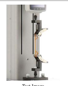
Test Image (GC-60: Rubber tape tensile test)
