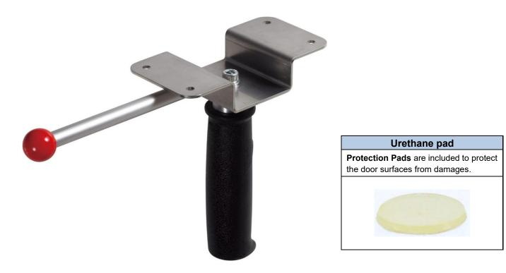
Specialized for fire door closing force measurement according to Article 112 in Enforcement Ordinance (amended in 2005) of the Building Standard Law of Japan.
