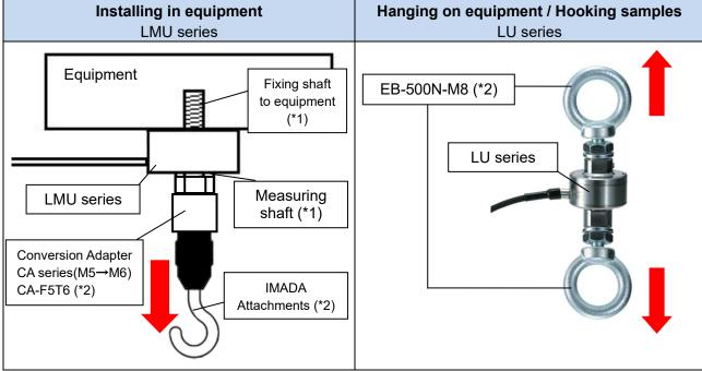
\*1 Fixing shaft and testing shaft look similar. Ensure the side is correct. Keep the space between the surface of the sensor and attachment or equipment using your own M5 nut.
