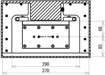
For MX2-500N, MX2-1000N, and EMX series, the mountable attachment length is 290mm. If you raise 5mm height of the test stand's table then the length can be 370mm.
