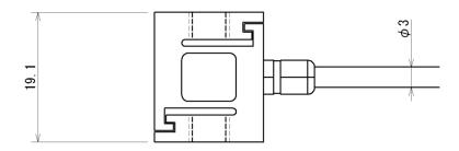
\* Do not screw in more than 3 mm as the sensor may be damaged.
