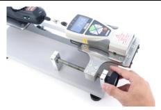
After adjusting the zero point and resetting to zero, turn the handles to hook each other's hooks and pull them together with the PSM and ZTA.
