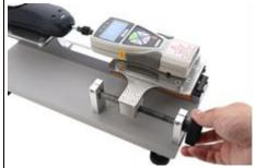
After adjusting the zero point and zero resetting, turn the handle to push the Flat Tips of PSM with that of ZTA.
