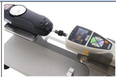
Check the accuracy of the ZTA by comparing the indicted force values on the PSM and ZTA.
