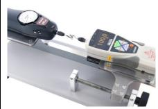
Check the accuracy of the ZTA by comparing the indicted force values on the PSM and ZTA.
