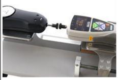
Mount the ZTA and PSM on the stand for the (push-force) measuring shafts facing each other. Attach the Flat Tip to the force gauge measuring shafts.
