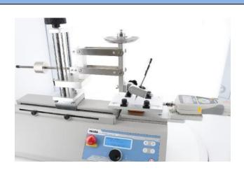
COF test of a pen using VWF-10N\*
