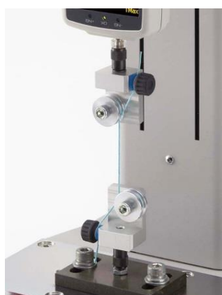
Test Image (Tensile test of fiber)
