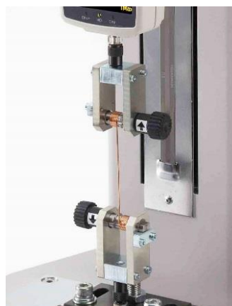
Test Image (Tensile test of copper wire)
