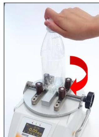
↑Opening PET bottle cap torque test
