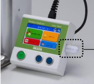
•Insert included USB flash drive into the controller.
