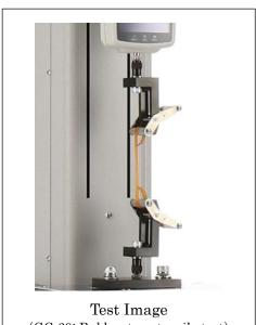
(GC-60: Rubber tape tensile test)
