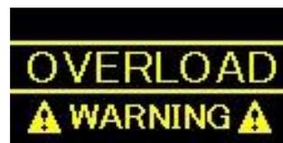
When load over its capacity is added, warning is indicated. Please stops measurement immediately when this indication shows up.
